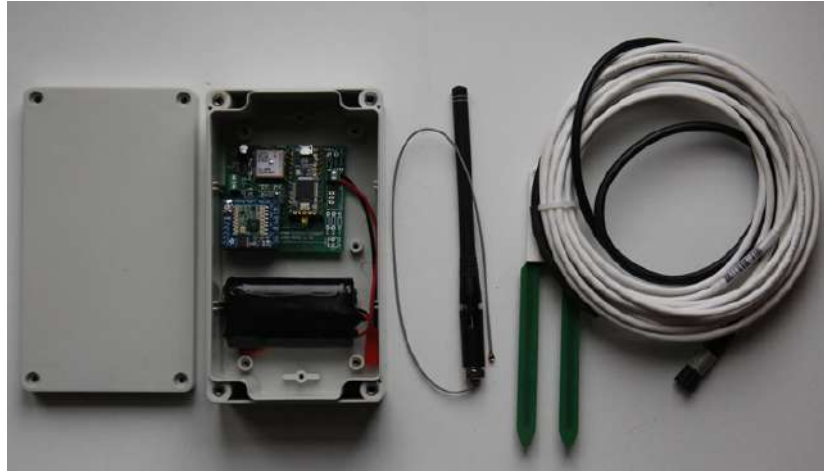
Figure 6 - Sensor of the LoRa network
