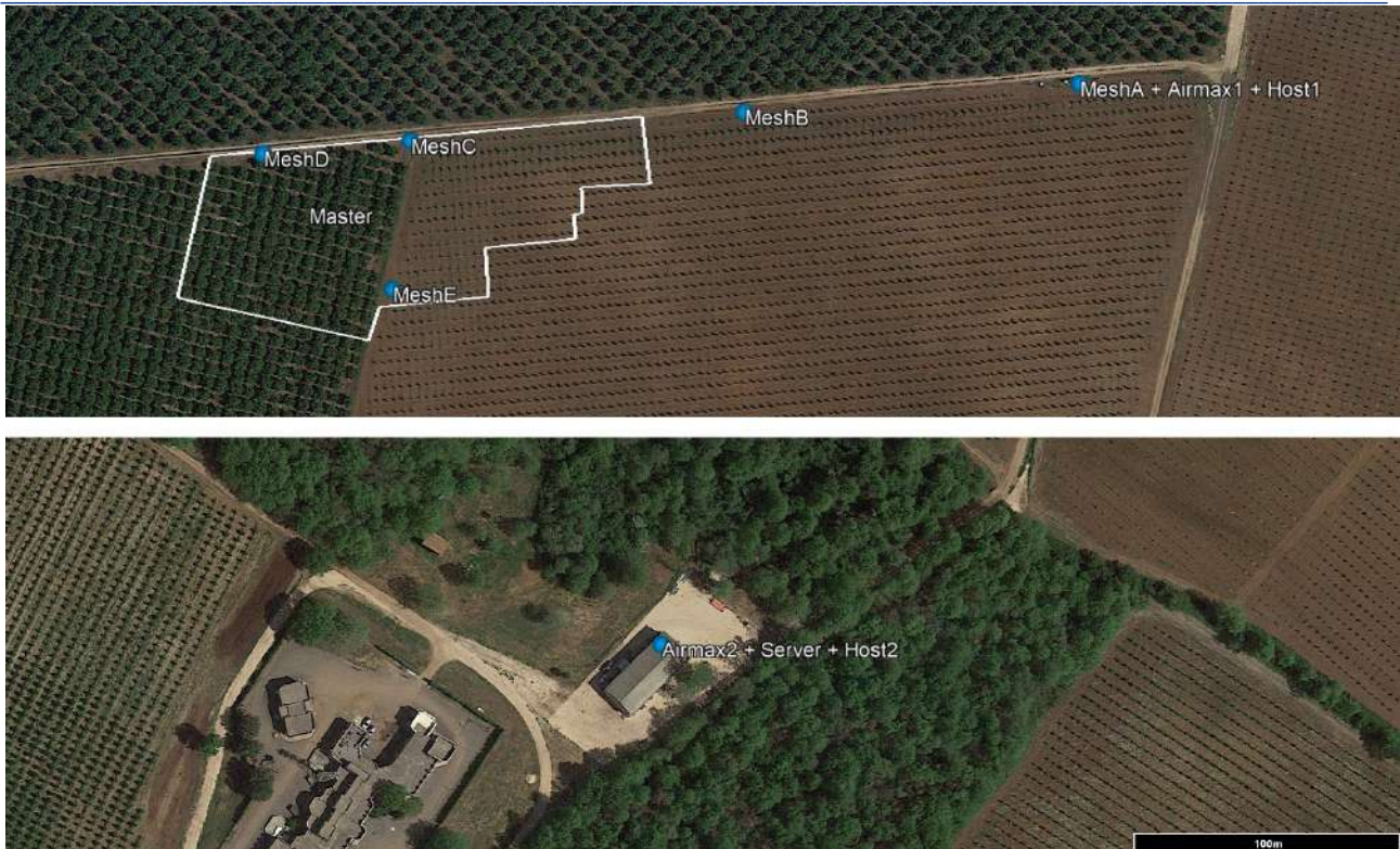
Figure 26 – Laptops location during RTT experimental test. The polygon describes the area where the “Master” was allowed to move
