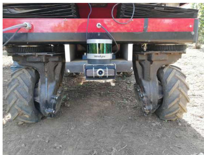
Fig. 2: Front view of the SHERPA HL robotic platform R-A with the Velodyne VLP-16 laser scanner and the Genius WideCam F100 webcam.
