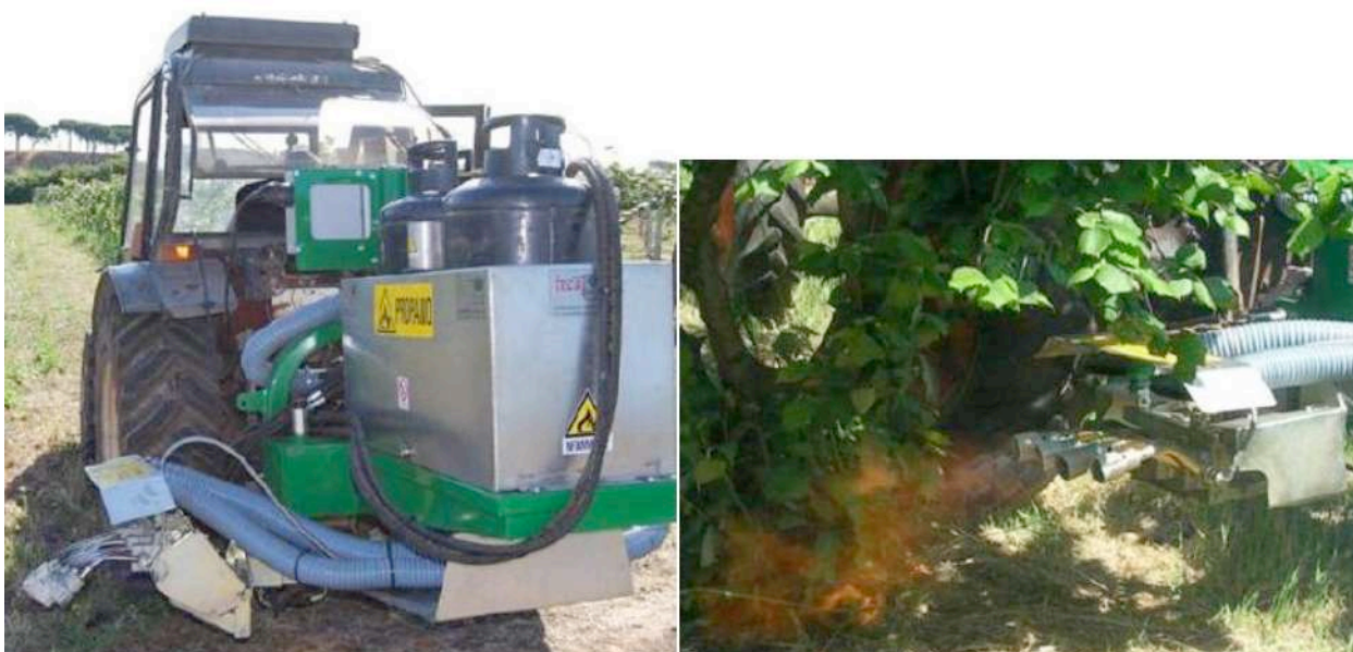
Figure 6 - Automatic “Orchard-Vineyard” pyroweed model (on the left) and automatic weeder field treatment tested on hazelnut (on the right).
