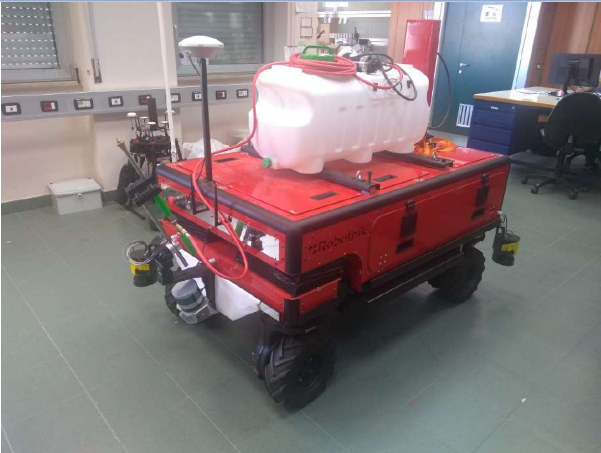
Figure 7 - UGV equipped to perform targeted application of chemicals on suckers.
