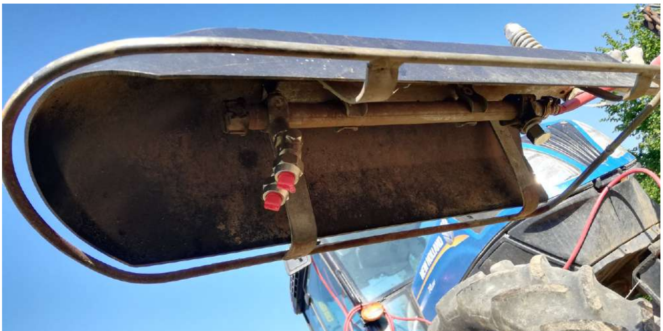
Figure 11 - Nozzles mounted on shielded equipment.
