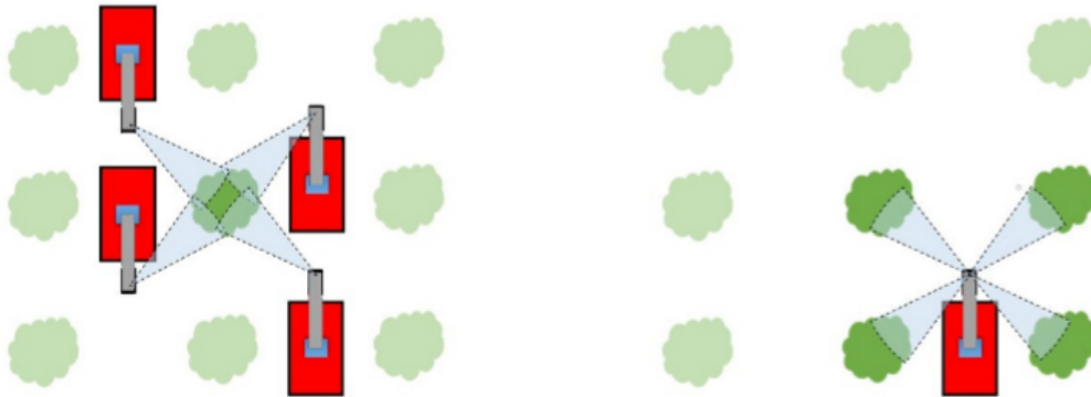
Figure 12 - Examples of scanning policies in a small patch of the target field. From left to right, the 4 scans that are necessary to 3D reconstruct the tree and the possibility on scan 4 different plants at the same location inside the orchard, respectively.
