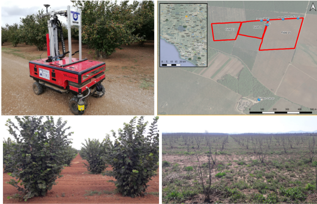
Figure 8 - On the top left, the SHERPA HL robotic platform prototype R-A, on the top right a satellite image on the experimental fields used in the PANTHEON project. On the second column, a hazelnut orchard in the harvesting and vegetation rest.
