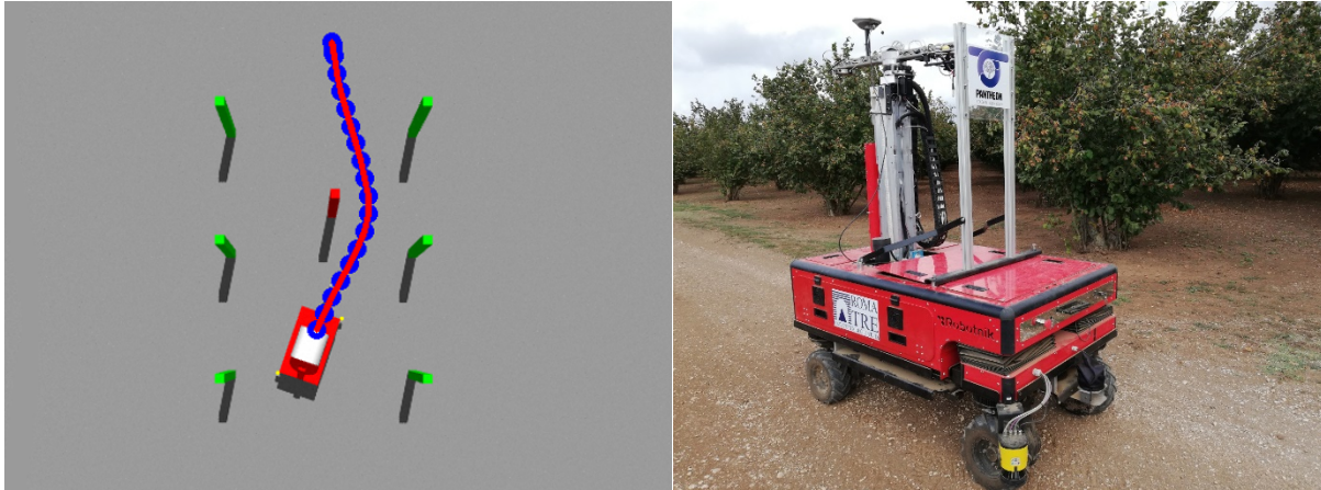
Figure 2 - Left: examples of a planned trajectory in a simulated scenario filled with static obstacles (green) and a dynamic obstacle (red). The green obstacles are arranged to resemble the planting layout of hazelnut trees as in the real field. Right: the SHERPA HL R-A robotic platform
