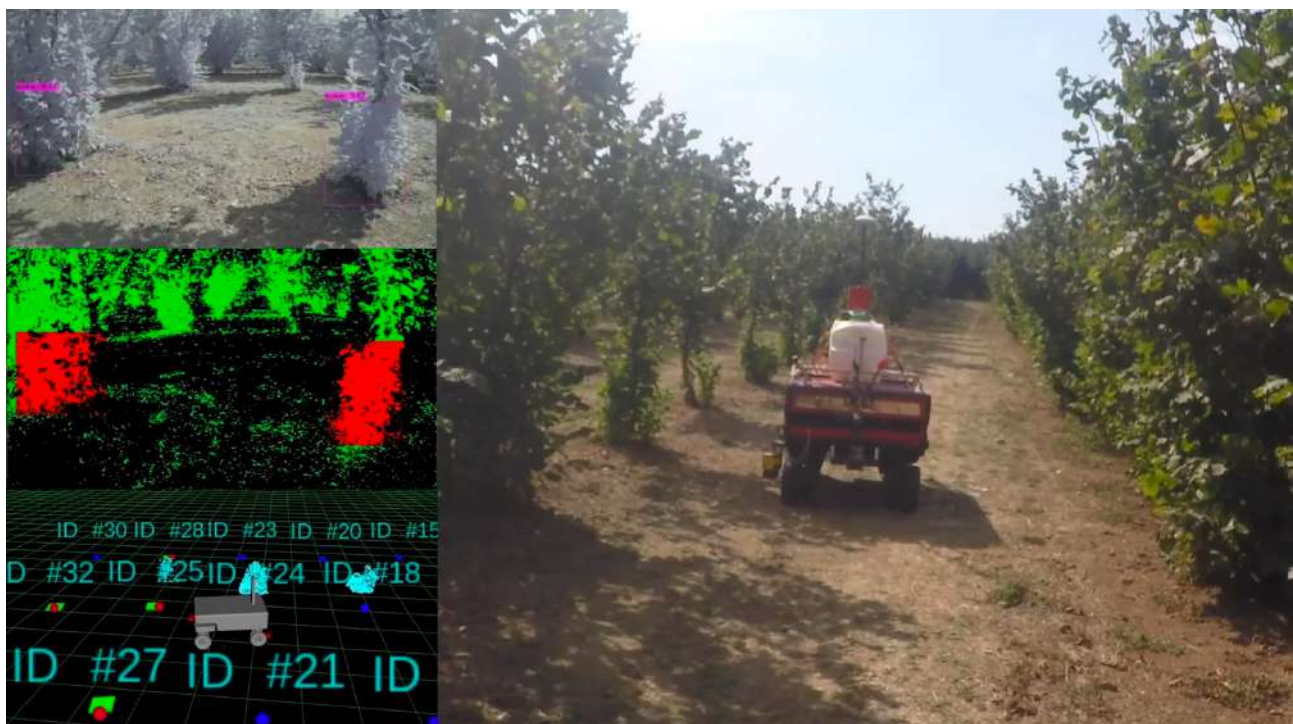
Figure 40. Real-time suckers' reconstruction conducted by the SHERPA HL R-B
