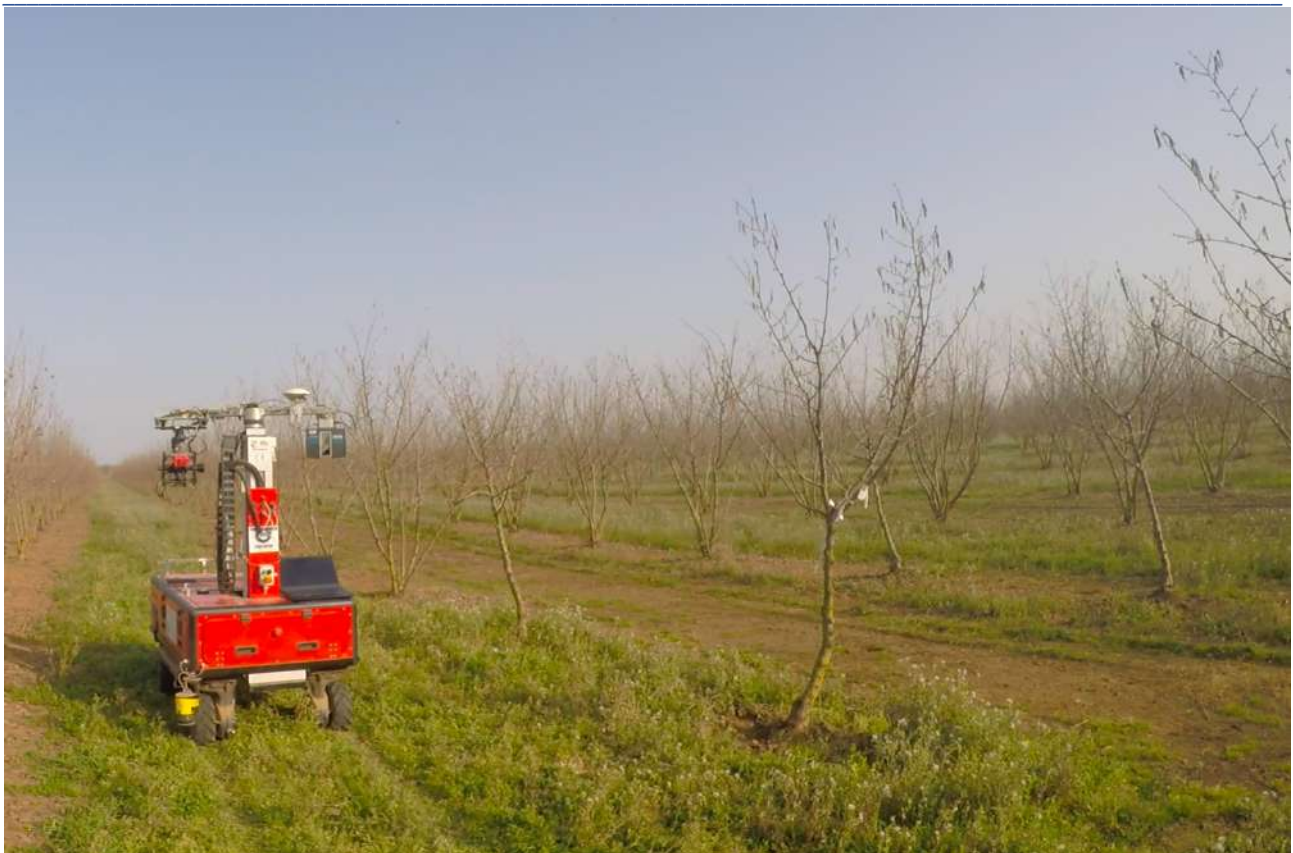
Figure 38. UGV acquiring data for the tree geometry reconstruction which enables the generation of the pruning suggestions
