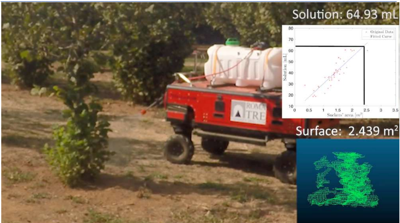
Figure 41. Application of the herbicide after the canopy area of the sucker has been estimated
